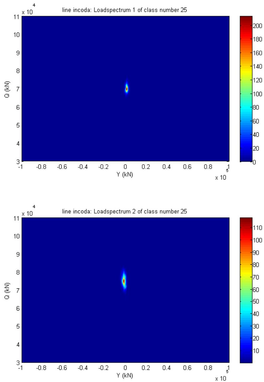
**Figure 5: Load spectra for class n°25 of Pendolino (rear bogie instrumented)**
