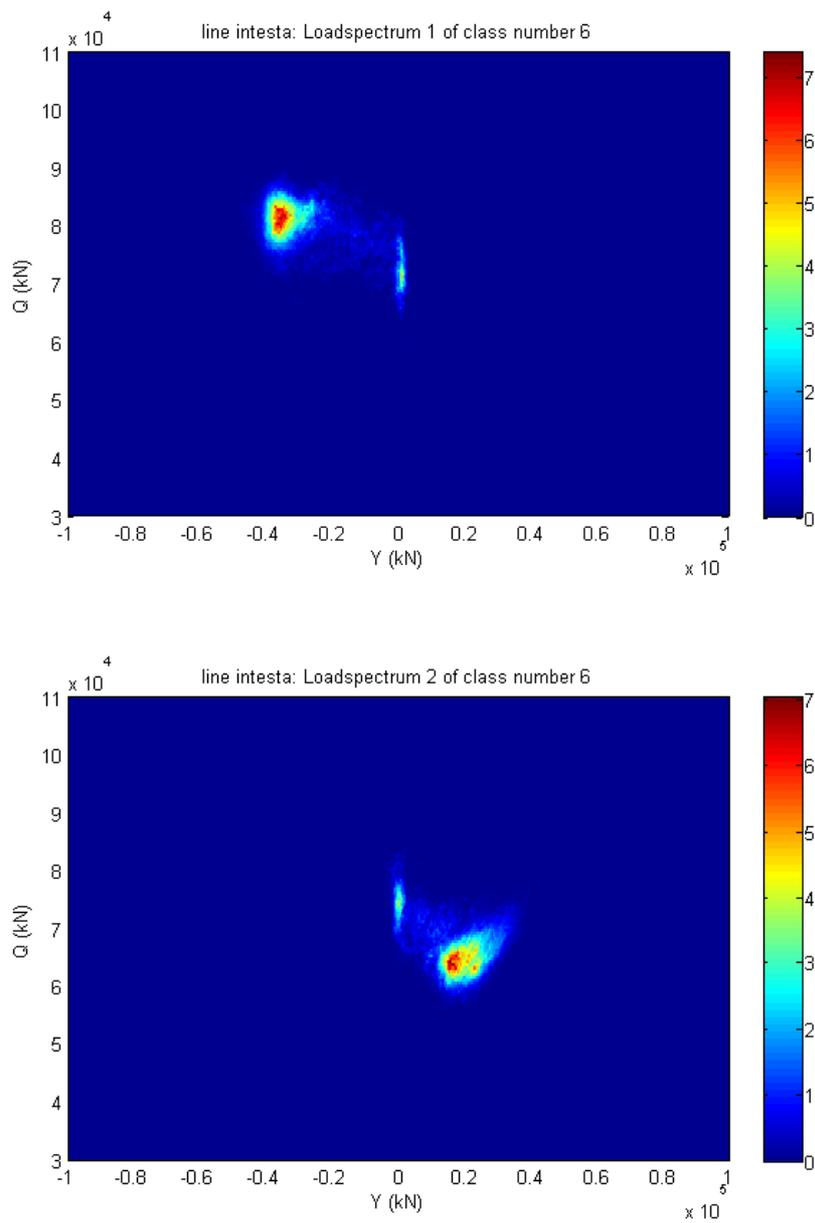
**Figure 4: Load spectrum for the Pendolino train (class number 6)**
