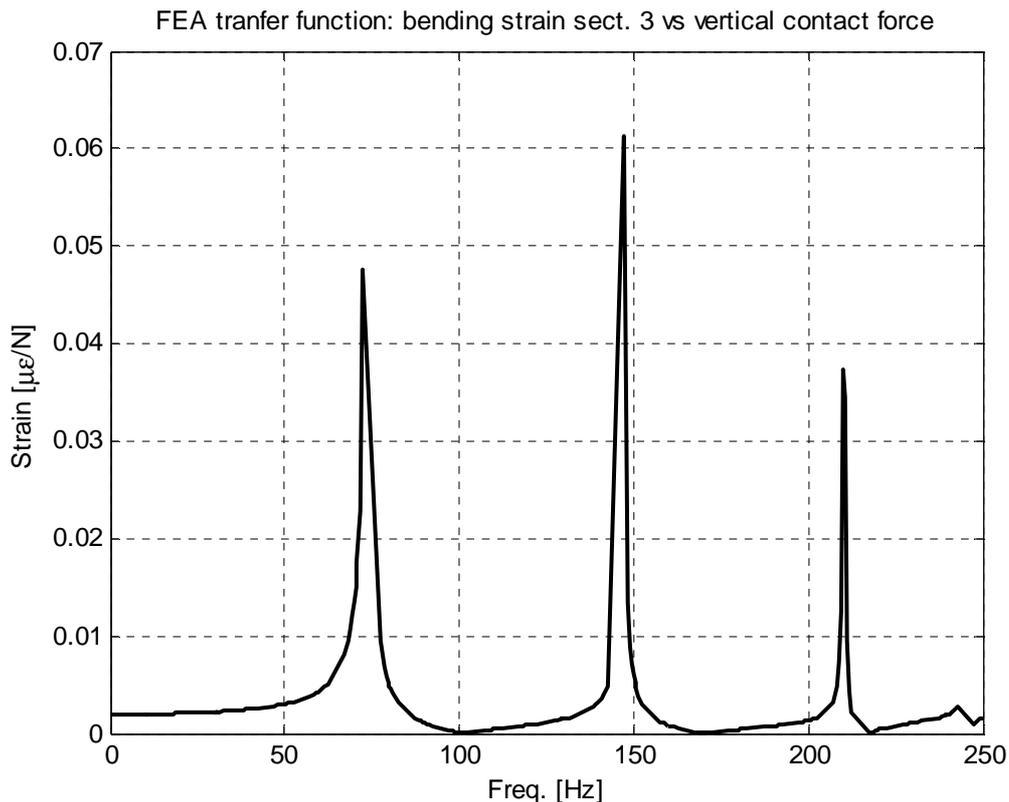
**Figure 1- Frequency response of the bending deformation in section 3 produced by a vertical force applied in the contact point, as obtained from a calculation performed on a finite element model of the wheelset.**
