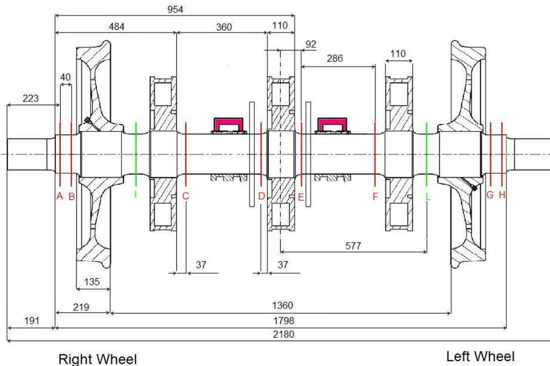
**Figure 2: Positions of the strain gages on the axle**
