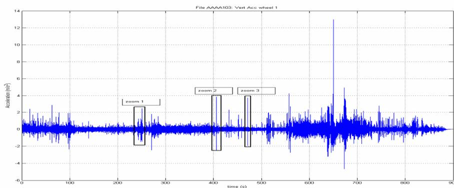
**Figure 1: Vertical acceleration in data file AAAA103 for the Pendolino**
