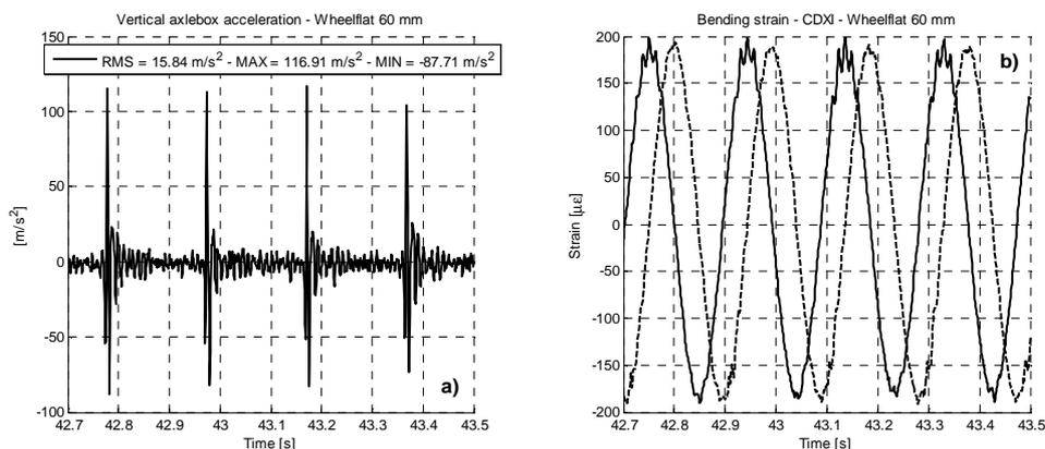
**Figure 4- Effect of an artificial wheelflat at speed 50km/h, measured on the Velim test circuit. (a) Time history of the vertical axle box acceleration. (b) Time history of the bending strain measured in section 3 of the instrumented wheelset.**
