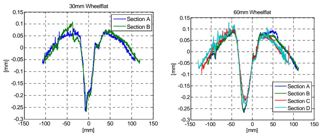
Figure 3- Circumferential measurements of the 30mm and 60mm artificial wheelflat.
