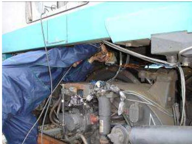
Figure 2- Execution of the artificial wheelflat on the measuring wheelset.
