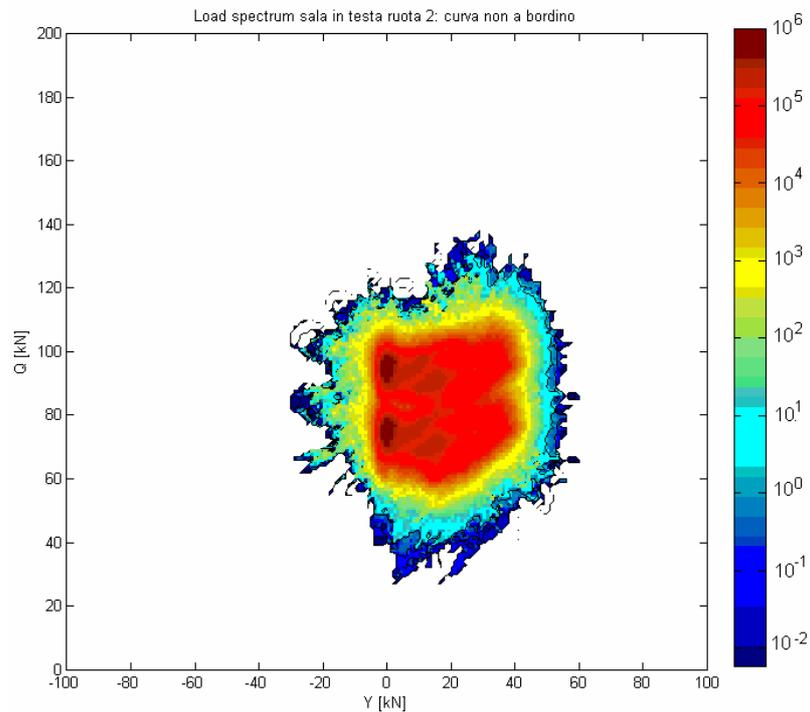
Figure11– Wheel 2 (leading wheelset) in curve not in flange
