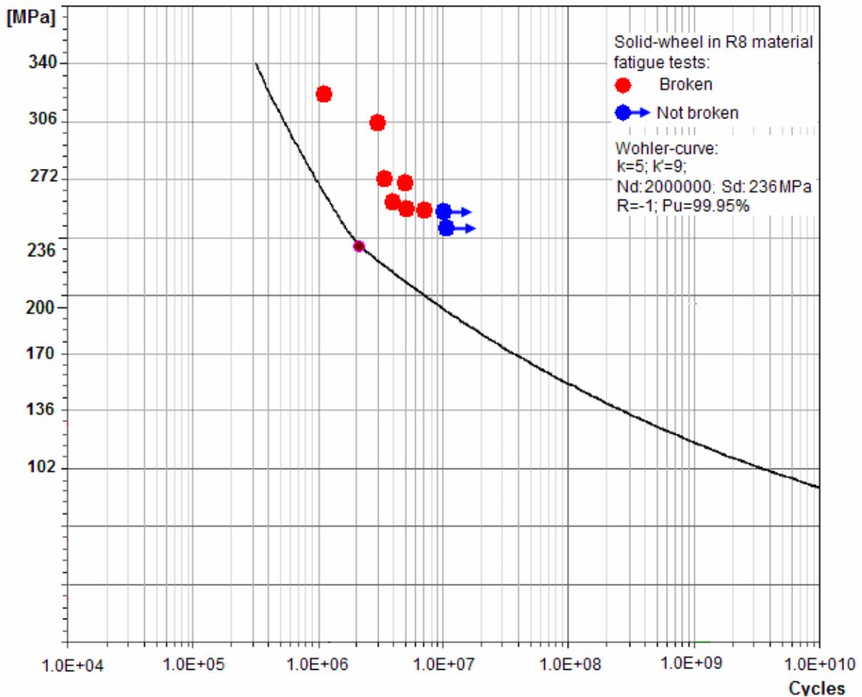
Figure 2 – Wohler-curve used in "Palmgren-Miner method"
