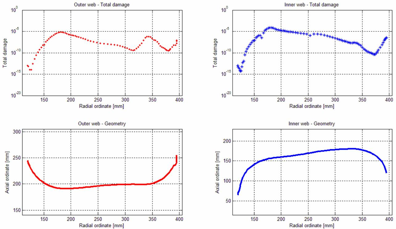
Figure 15– Total damage fraction for the web (the inner part in bleu and the outer part in red) of the original wheel
