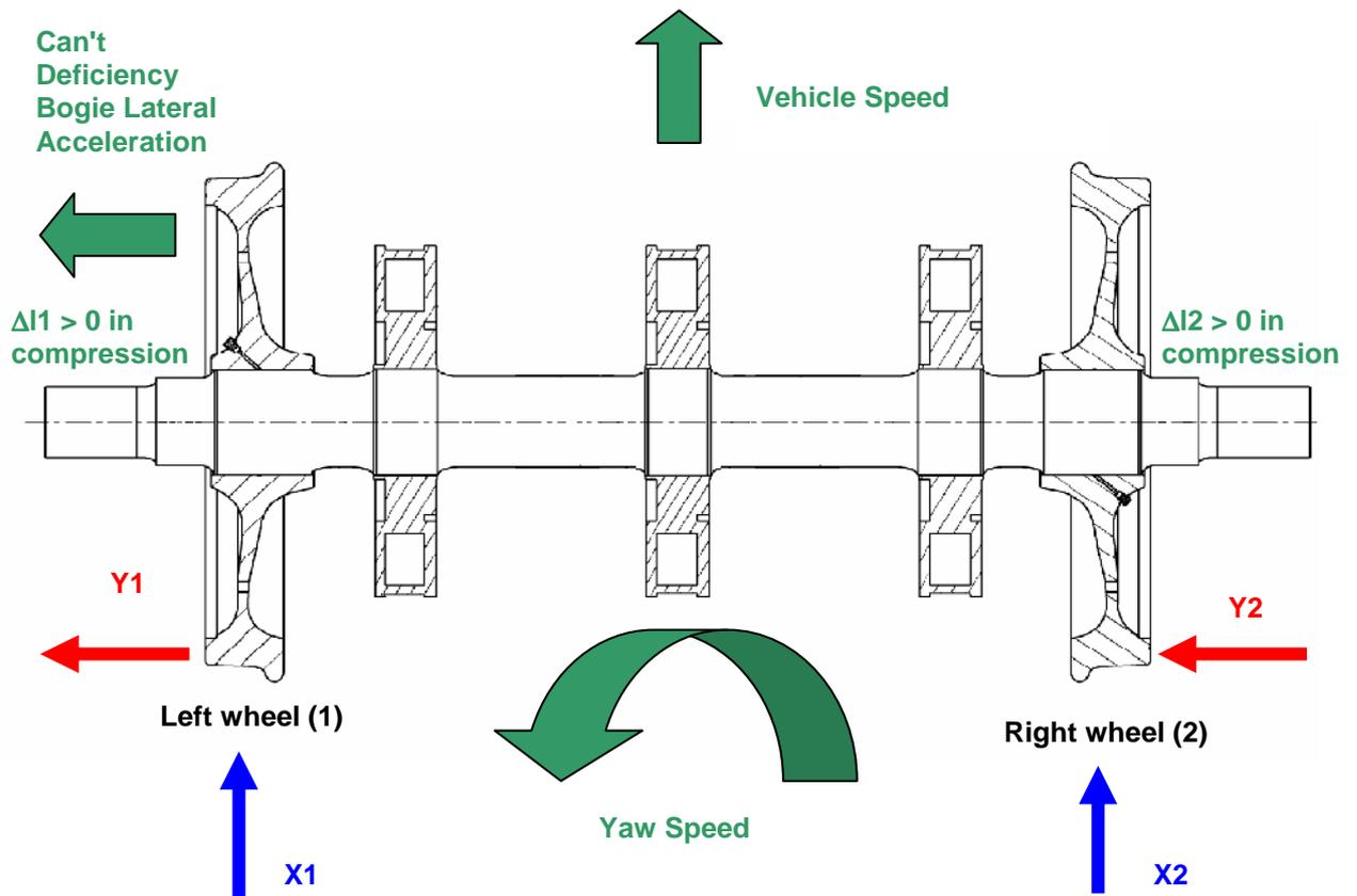
Figure 3 – Convention for the versus of spectra loads
