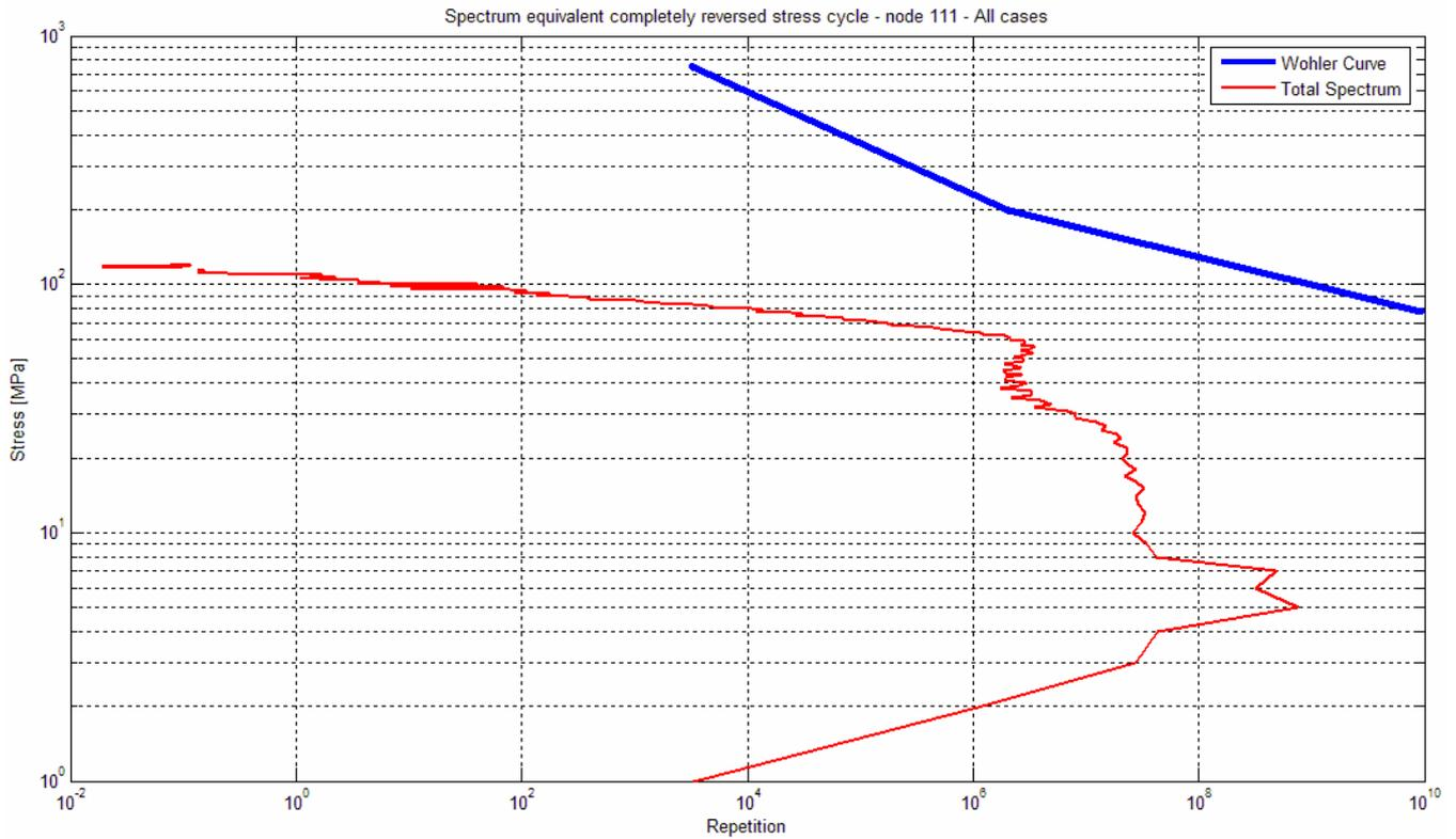
Figure 16 New wheel with 10% less mass; stress spectra for most critical node;
