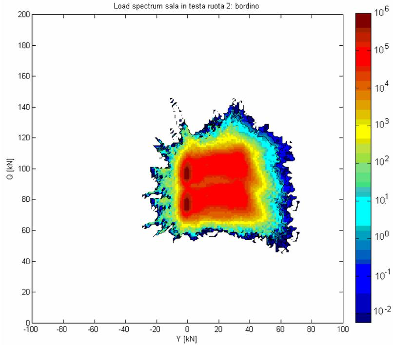
Figure10– Wheel 2 (leading wheelset) in curve in flange
