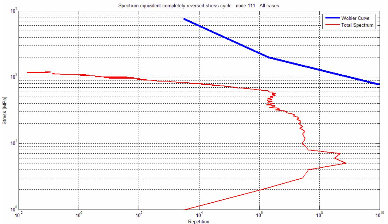
Figure 14 Original wheel; stress spectra for most critical node; Wohler curve for R8T
