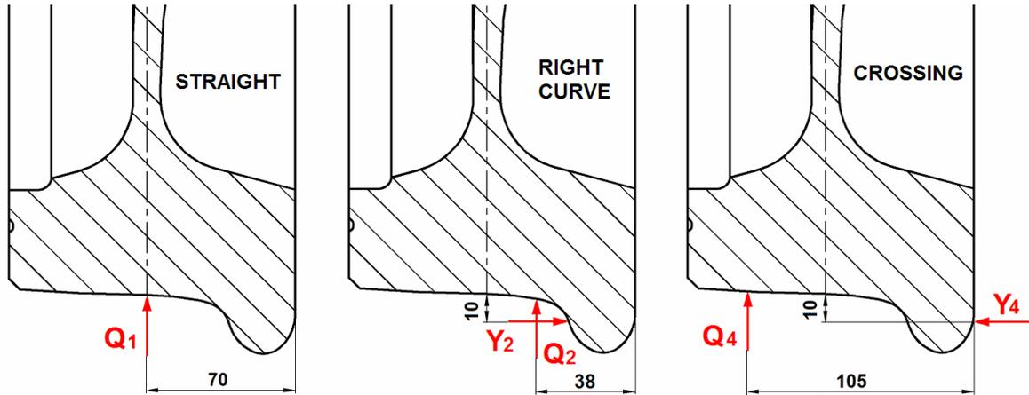
Figure 1 Position and direction of application of the forces according to UIC 510.5
