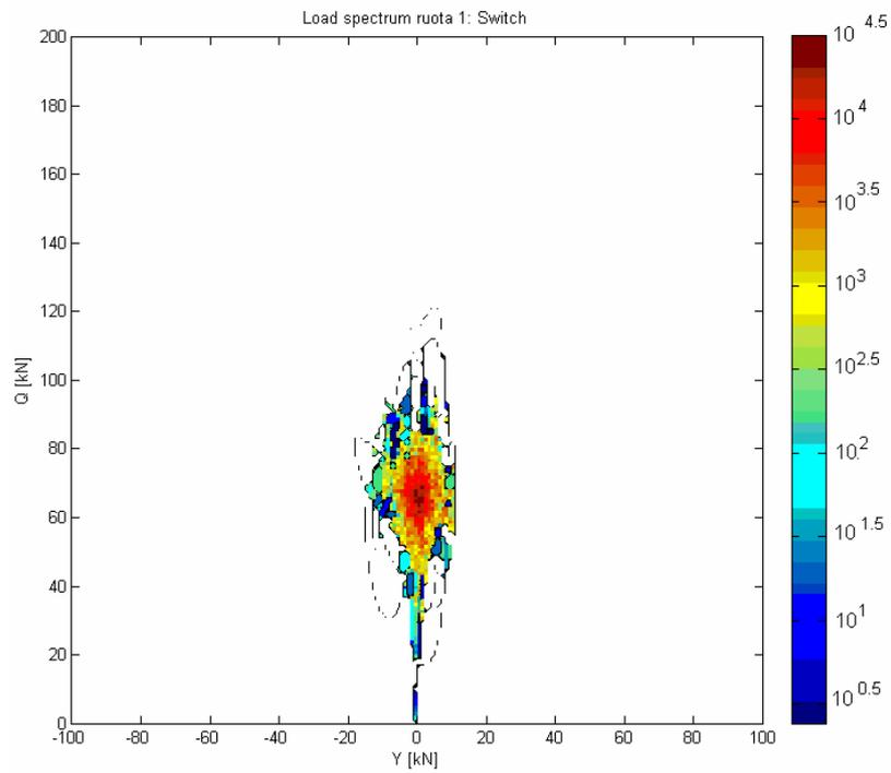
*Figure 8 – Wheel 1 over switch*
