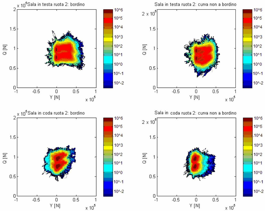
Figure 9 – Load spectrum for wheel 1, leading wheelset and trailing wheelset in curve
