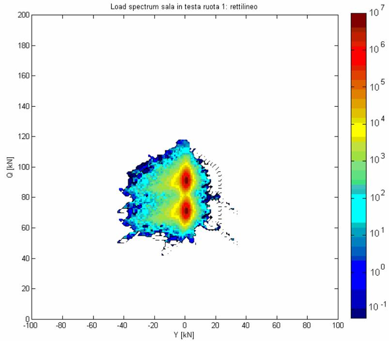
*Figure 7 – Wheel 1 (leading wheelset) in straight running*
