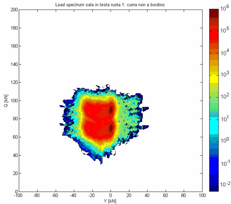
Figure 6 – Wheel 1 (leading wheelset) curve not flange
