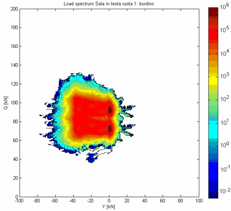
Figure5 – Wheel 1 (leading wheelset) curve in flange
