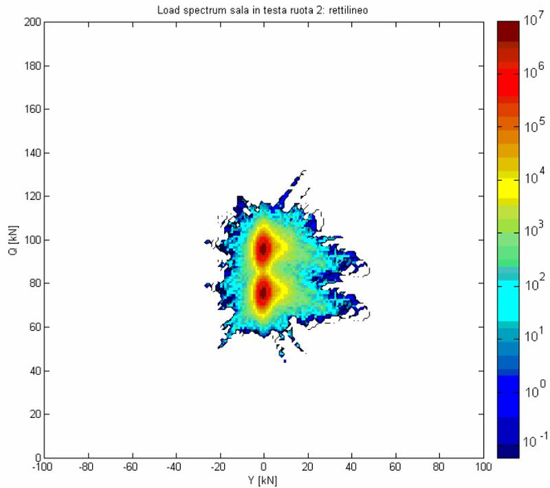
Figure 12 – Wheel 2 (leading wheelset) in straight
