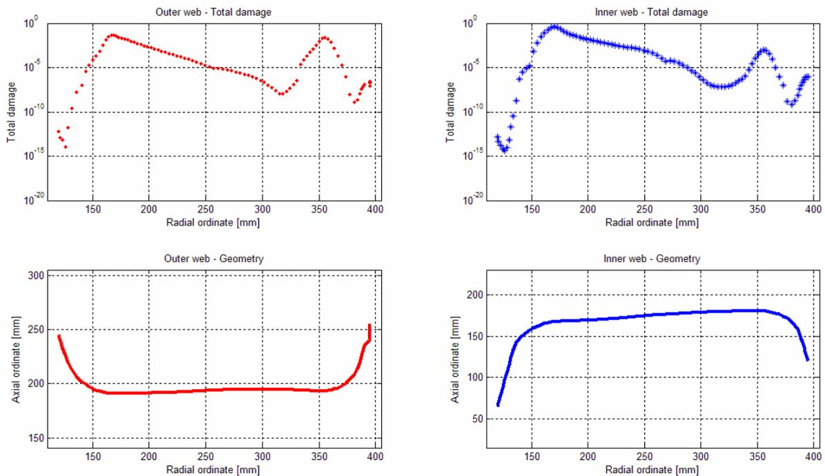
Figure 17 – Total damage fraction for the web (the inner part in bleu and the outer part in red) of the new wheel
