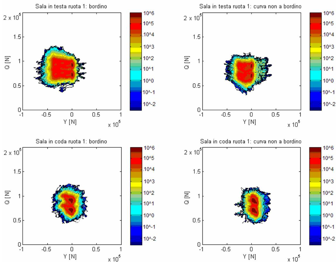
Figure 4 – Load spectrum for wheel 1, leading wheelset and trailing wheelset in curve
