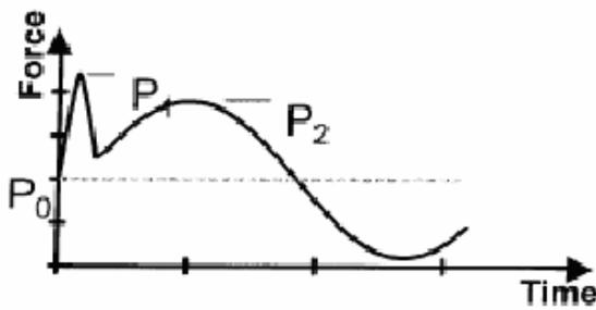
$P_0$  is the static load of the wheel,  $P_1$  the first peak which appears in the gradient discontinuity is the wheel rail effort taking into consideration the herzian stiffness and  $P_2$  the second peak taking into consideration the track stiffness including rail, sleepers and ballast.
